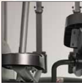
Rollmentum™ Center-Drive System features guide rollers which provide maximum bearing life.
