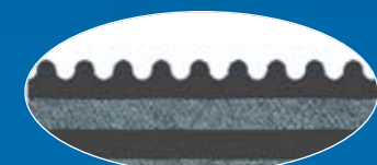
Standard 4-ply treadbelt 5X magnification
