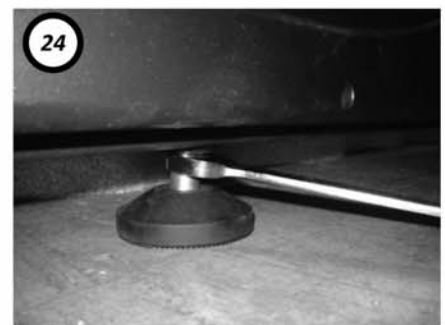
24 Check stability of unit by verifying that all leveling feet are pressing against the floor.
