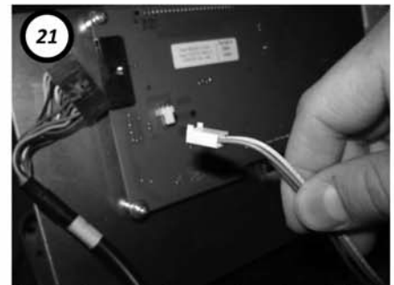
21 Connect the upper harness from the upright to the edge connector and the accessory harness coming from the POD to the 3-pin connector.
