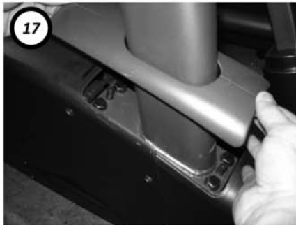
17 Install the Upright Mount Covers. Screw the outer and inner pieces together trapping the upright and slide them down until they click.
