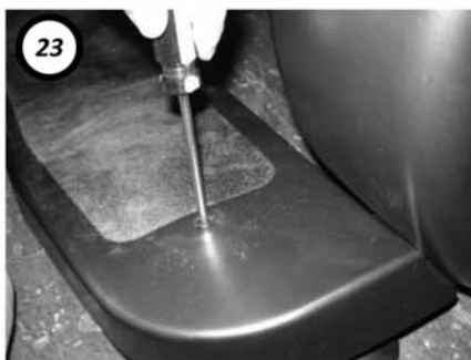
23 Install the rear step with 2 phillips screws (L).
