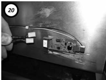
20 Connect the 2 heart rate cables to the 2 side by side 3-pin connectors on the small PC board on the far side of the membrane.
