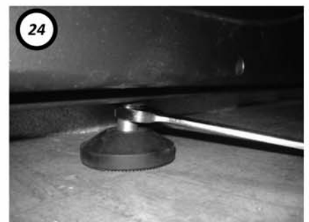
24 Check stability of unit by verifying that all leveling feet are pressing against the floor.
