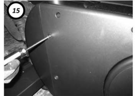
15 Install the Base Endcaps using 4 phillips screws (I) for each. * If installing an LVS (optional), go to those instructions now.
