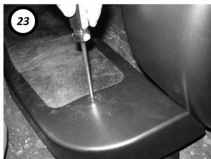
23 Install the rear step with 2 phillips screws (L).
