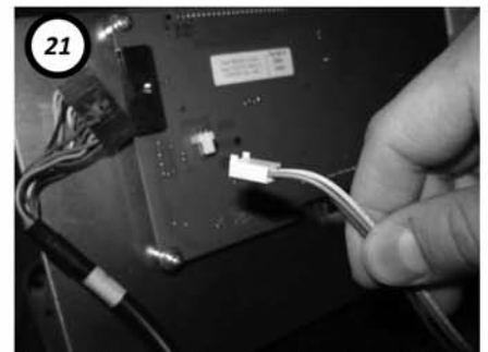
21 Connect the upper harness from the upright to the edge connector and the accessory harness coming from the POD to the 3-pin connector.
