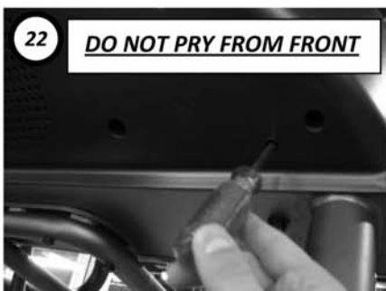
22 DO NOT PRY FROM FRONT Press membrane into set position. If you need to free the membrane, use a long screw driver to pop it out from back using the access hole.
