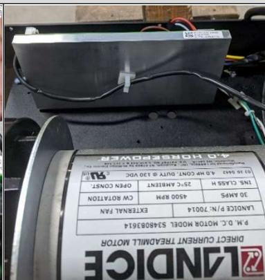
Braid the White/Black motor wires and secure it to the motor pan. Then route the drive motor wires to the lower board, ground the green wire to the motor pan. Route the Speed Sensor wire along the back of the lower board, securing it in the clip, or with electric tape to the back of the lower board.
