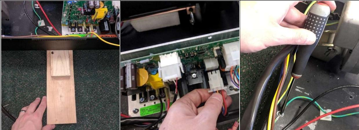
Begin by using a block of wood or something sturdy that can be propped underneath the motor pan. You will then power down the unit, and unplug from the power source. Next, locate the elevation harness and unplug from the lower board. Finally, use your screwdriver to remove the grounding wire.
