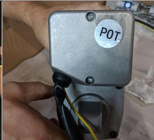
For new Landice units, the elevation pot key will be located in the motor pan, as shown above. If replacing an elevation motor on an older unit, the key will be bound along the grounding wire. **NOTE: Needle nose pliers can be used in the event the pot key is lost.** Remove the POT sticker to expose the elevation pot and proceed to the next step.
